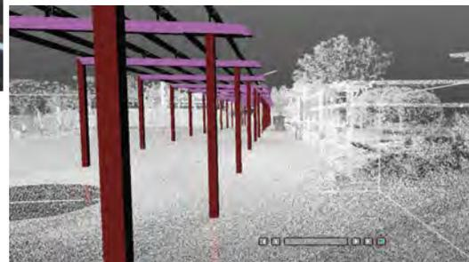
“ Using our 3D Scanning Technology and Robotic Total Station for site measurement, we were able to overcome the challenges of this project, which included uneven ground level and footings designed at varying heights. The accuracy of this technology enabled a seamless flow from measurement through to fabrication & installation, allowing us to complete the job within time-frame with no rectification works. ”
