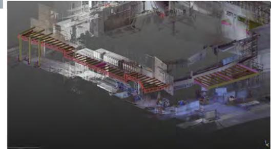
*Using the 3D Laser Scanner to scan each section of this job, we were able to identify all potential clashes between the existing site and our shop drawings. This made the entire construction process simple, effective, and efficient.*
